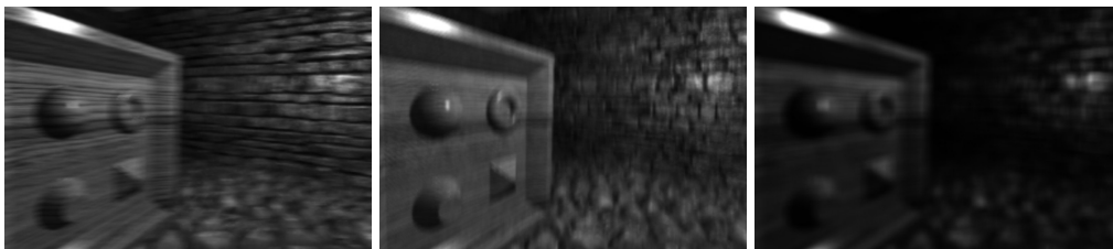
Figure 10: Bloom intermediate images: (a) horizontal blur, (b) vertical blur, (c) composed final blurred image to be added to final scene for bloom effect.
