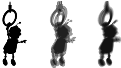
Figure 10: Combining several occlusion maps to compute soft shadows. Left: the occlusion map computed for a single sample. Center: the attenuation map computed using 4 samples. Right: the attenuation map computed using 64 samples.
