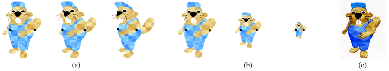
Figure 9: (a,b) Our particle method illustrated with a chessboard texture. (a) Rotation: 2d textures follow 3d particles (black dots), (b) z-translation: An infinite zoom of the texture maintains a constant frequency. (c) Result when using our pigment and paper textures.
