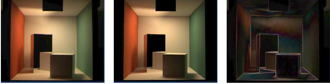
Figure 1.5: Measured, simulated and error images of a scene. This famous scene, called the Cornell Box, was setup by researchers in Cornell University’s Light Measurement Laboratory. The potential for multiple interreflections between diffuse surfaces and the availability of measured parameters of illumination of reflection made this scene a popular choice for verifying global illumination algorithms. (Source: Cornell University Light Measurement Laboratory)
