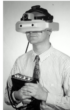
Figure 2: The Vision Enhancement System developed by Massof et al. allows patients that suffer from macular disease to perceive a high contrast version of the world, with style.
