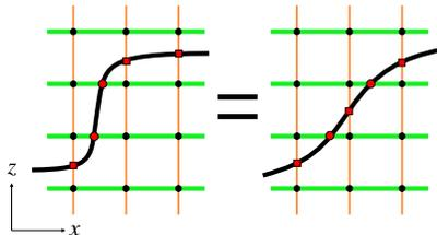
Figure 2: A step variation and a smooth one are equivalent in the uniform region: they cross the same number of  $x$ -edges (2 circles) and  $z$ -edges (3 squares). For clarity purpose, we present a 2D  $xz$  plane of the 3D grid.
