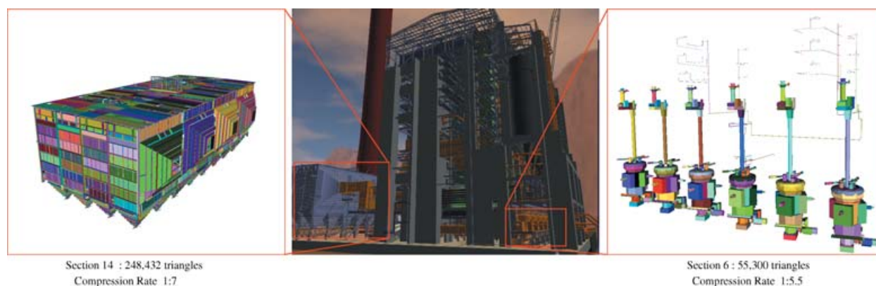
Fig. 12. Detecting symmetries and similarities between tiles created from a raw list of polygons allows us to compress geometric models in two ways: (1) by instancing similar tiles and (2) inside each symmetric tile, by instancing the part of the geometry which permits to reconstruct the whole tile. In such a big model as the powerplant (13 millions triangles), we achieve a compression ratio (ratio of geometry file size in X3D format) of 1:4.5. We show in this figure two subparts of the complete model. For each, we show the tiles computed by our heuristic (see Section 6.5) as well as the obtained compression ratio. The PowerPlant model is a courtesy of The Walkthru Project.
